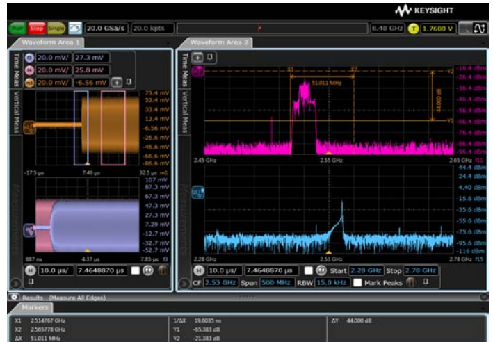
Perform measurements in the area of interest through the gated function.
